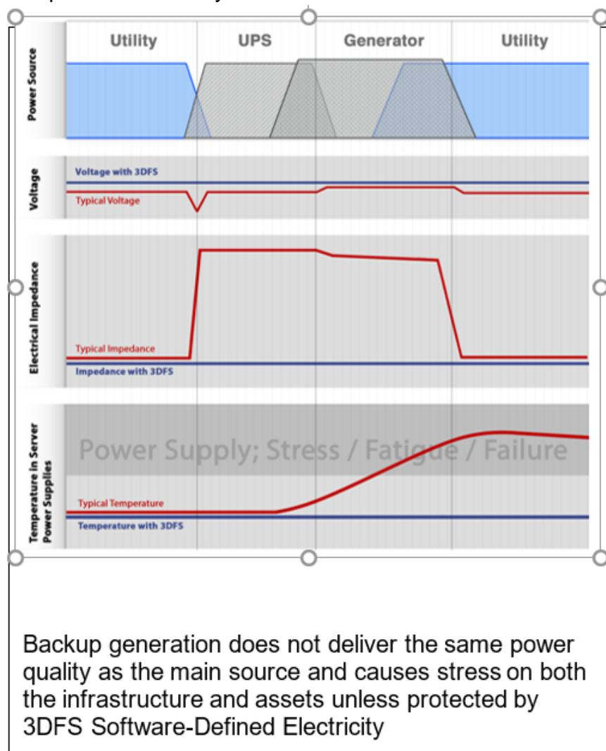
Figure 5: Effect of Variance in Impedance/Voltage on Server Power Supply
