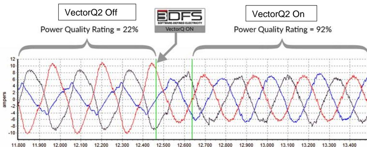
Figure 3: SDE VectorQ2 Detection and Correction of Energy Events
